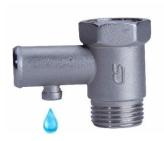
When the pressure in the system is increased due to the operation of the water heater safety valve, the water is discharged from the valve discharge nozzle in the form of droplets. **This is a sign that you are in safe, and this is definitely not a negative situation.** In this case, what needs to be done is to connect an 8 mm hose to the drain mouth and connect the other end to a drain.
