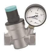
The dripping of the water heater safety valve is extremely natural and safe when the water in the boiler is hot. If the vent is dripping while the system is cold, check the network pressure. If you observe the mains pressure is high, it is advised to install the water pressure reducer with manometer to reduce this pressure to the desired level.
