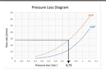
The graphic is prepared according to the conditions specified in EN 1567 standard. (Input pressure 8 bar - Output pressure 3 bar)
