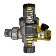
Automatic Filling Valve is connected to the water inlet line in closed circuit heating systems. It is a device consisting of pressure reducer, shut-off valve, check valve and filter. It provides automatic completion of the water that has decreased in the system.
